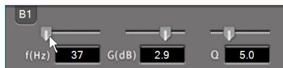
Example of IIR pole adjustment
