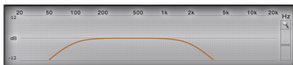
Crossover frequency 80 - 2000 Hz @ 12 dB/Oct.
